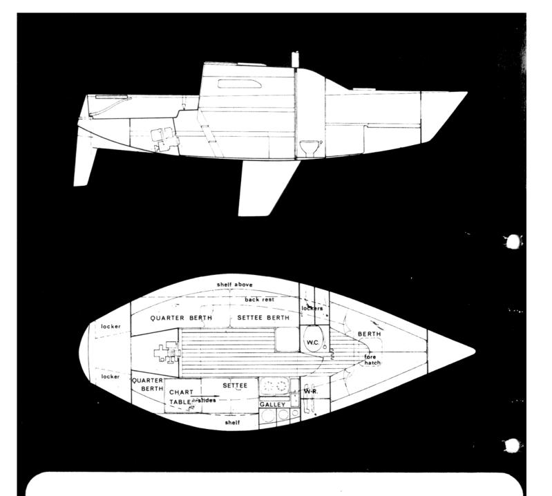
'EYGTHENE 24' a new and stimulating design with a proven offshore racing performance and comfortable cruising ability.
